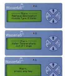
The microprocessor will provide with a preventive notification, in the form of an audible warning and a written message on the screen, indicating the maintenance tasks required to guarantee the desired water quality.
